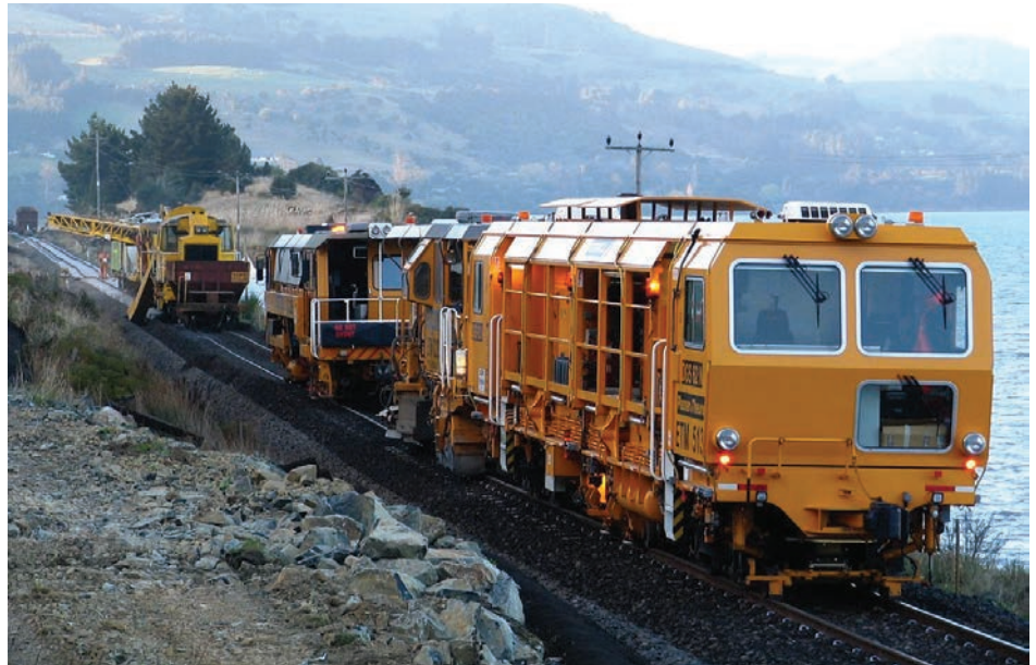
A dynamic track stabiliser. Photo: KiwiRail
